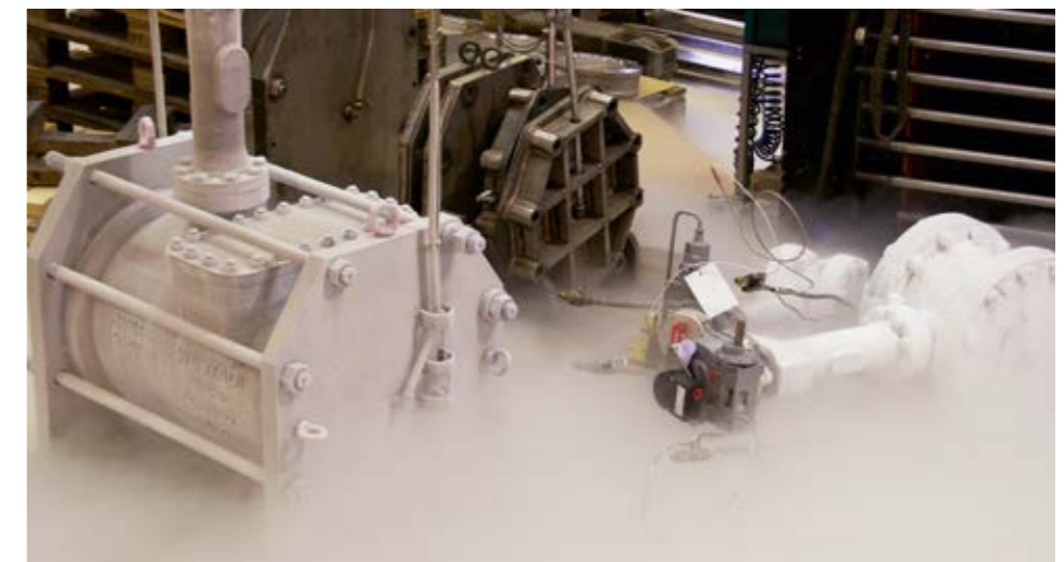
A cryogenic butterfly valve undergoes testing at -192 °C
